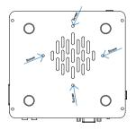
Using the supplied M3 stand-off screws, follow the reference above. Once complete, lock into the VESA Mount.
