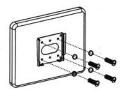
Place 4 screws through the Tablet Mount Part and fit this onto the Tablet.
