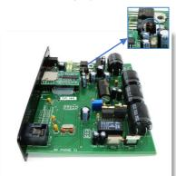
2. Move the jumper from its original position on the right (5V) to the 12V position on the left.
