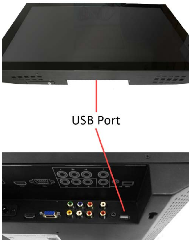
Figure 1 Position of screen inputs
